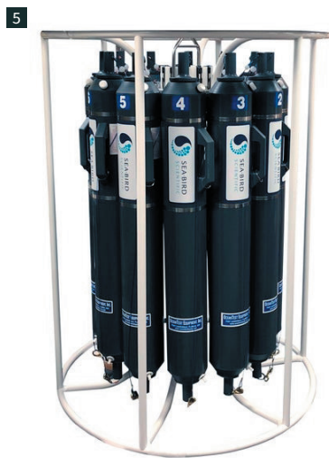
1 Oceanographic winch 2 Wetlab 3 Pyranometer, 4 PCO2 5 Rosette, Carousel Water Sampler 6 Tube TVO moonpool 7 Inertial measurement 8 Scientific echosounder EA440.
