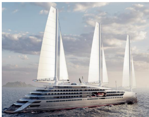
As part of the call for tenders process, two sail propulsion systems are being considered. Here is a 3D image of Swap2Zero with Solid Sail technology.
