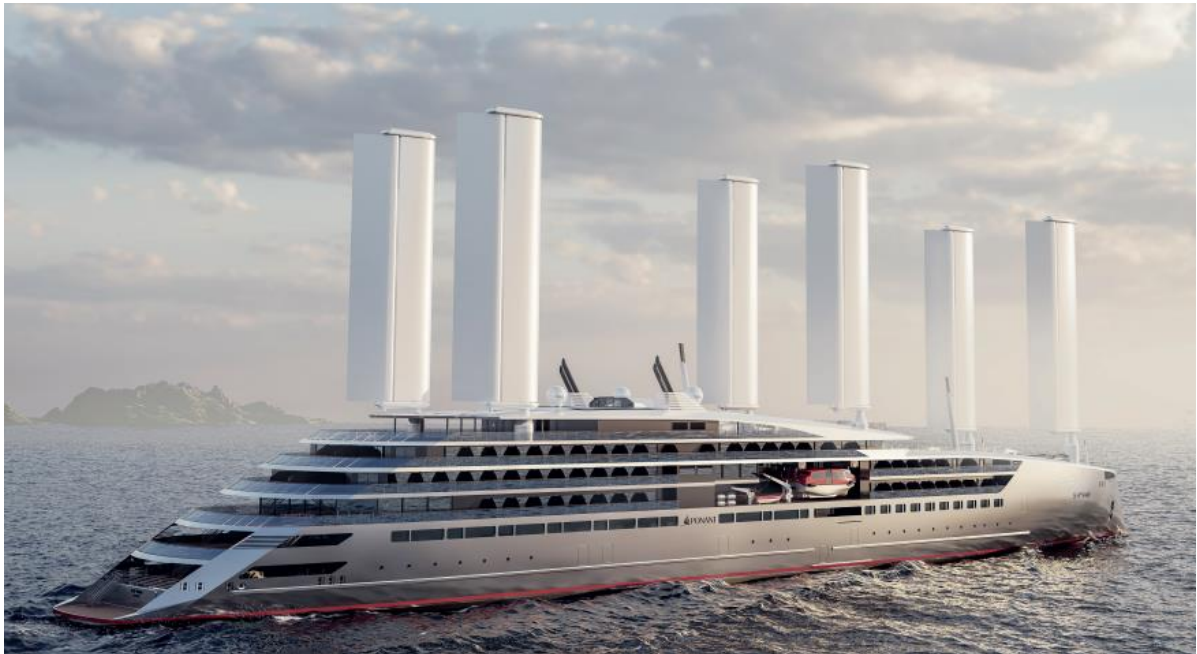
3D image of Swap2Zero project. In the call for tenders process, two sail propulsion systems are being considered, above is Ayro Oceanwings® technology.
